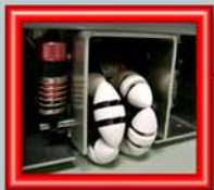
The front bi-directional wheel with dampers.
